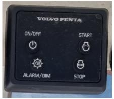
Should you hear an engine alarm during operation, check the tachometer to identify the reason for the alarm (over heating/oil pressure/battary) immediately shut down the engine-CALL Technical support.
