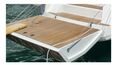
Attantion: Keep the platform closed while sailing, as well as in the anchor, when a high wave hits the platform. Otherwise, the platform would be damaged. only two people on platform is acceptable.
