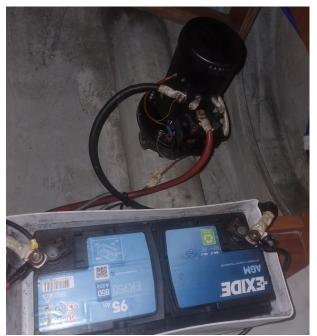
Remote control of bowthruster Quick (maximum time of continuous operation 5 seconds).
