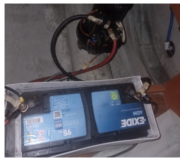
Bowthruster battery and fuse located under the bed in starboard bow cabin
