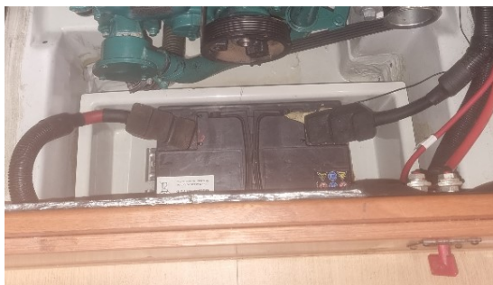
Engine battery and switch located in front the engine under the companionway ladder
