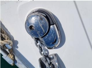
Remove the safety line and push the anchor over the bow, keeping hands and feet clear. Control the rate the chain pays out by tightening or loosening the brake with the windlass handle.
